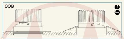
Professional Downlights are available in trimless and flanges recessed models, both in three different diameters: 55mm, 75mm, and 95mm,
